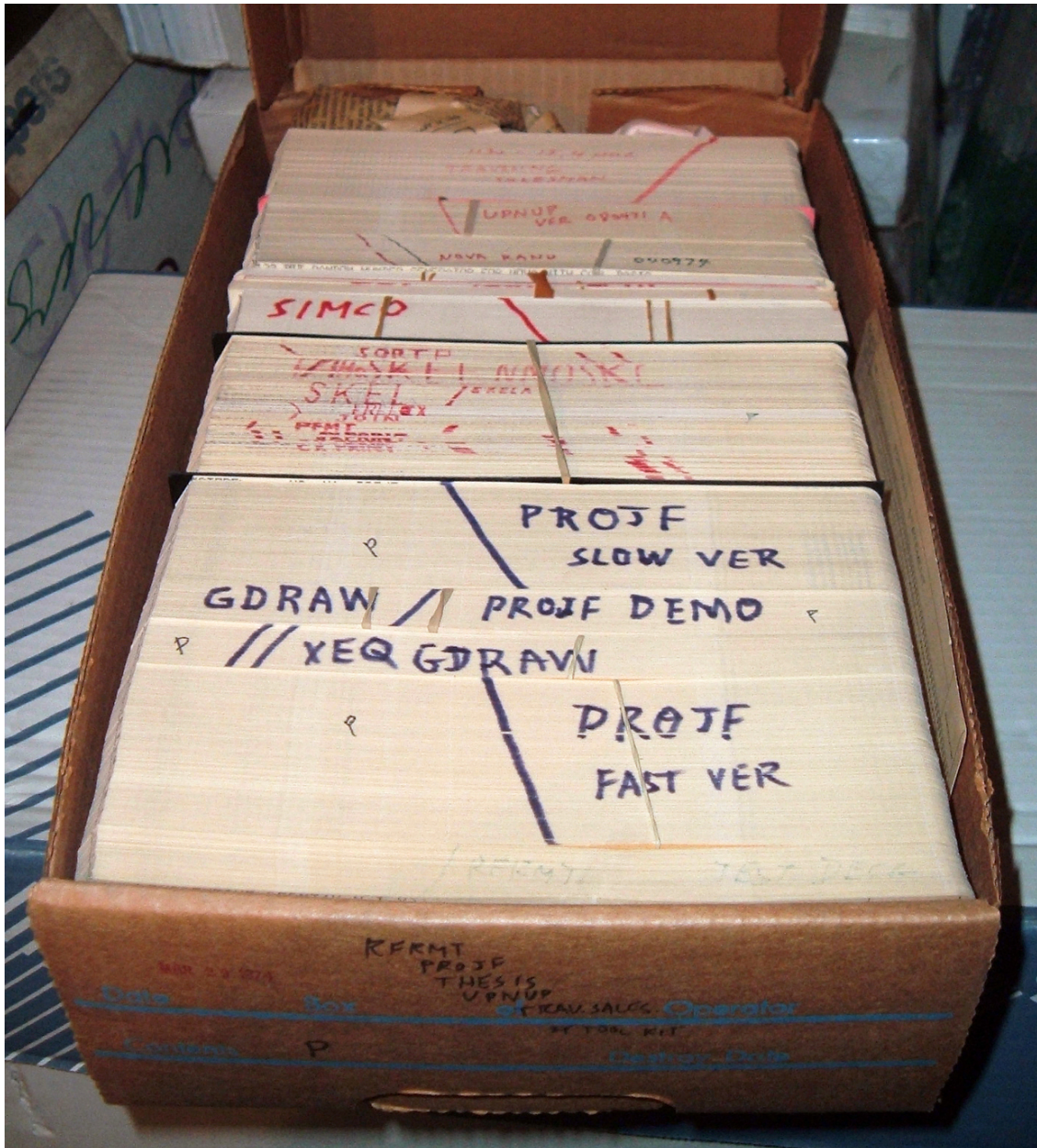
Figure 27 Data and instructions could be stored on external punched cards, which were kept in order and arranged in program decks.
