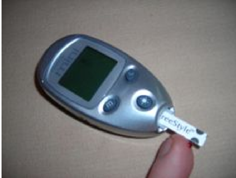
Figure 19.8: A person with diabetes has to monitor their blood glucose carefully. This glucose meter analyses only a small drop of blood. For an animation of diabetes Diabetes Cause and Effect , see ( http://video.google.com/videoplay?docid=6553371894741533041&#38;ei=Q4k6SoTVJIGEqAOK0fj_Aw&#38;q=diabetes&#38;hl=en&#38;client=safari ). (1)
