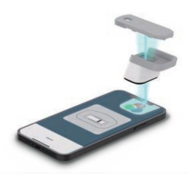
PixoTech® as iXensor's core technology platform can turn smartphones into in vitro diagnostic (IVD) devices. It utilizes the lighting and image sensing modules of the smartphone to detect the color change reaction on the immunoassay or colorimetric strip. The images of the test strip are captured by the front camera of the smartphone and analyzed via the proprietary algorithm to turn out a qualitative or semi-quantitative, or quantitative result.
